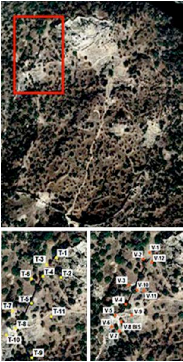
Figure 3. Study zone and location of the scanner stations (V-i) and targets (T-i) for georeferencing.
